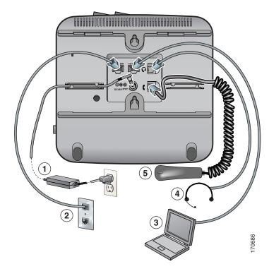
Figure 3-1 Cisco Unified IP Phone 7931G Cable Connections
